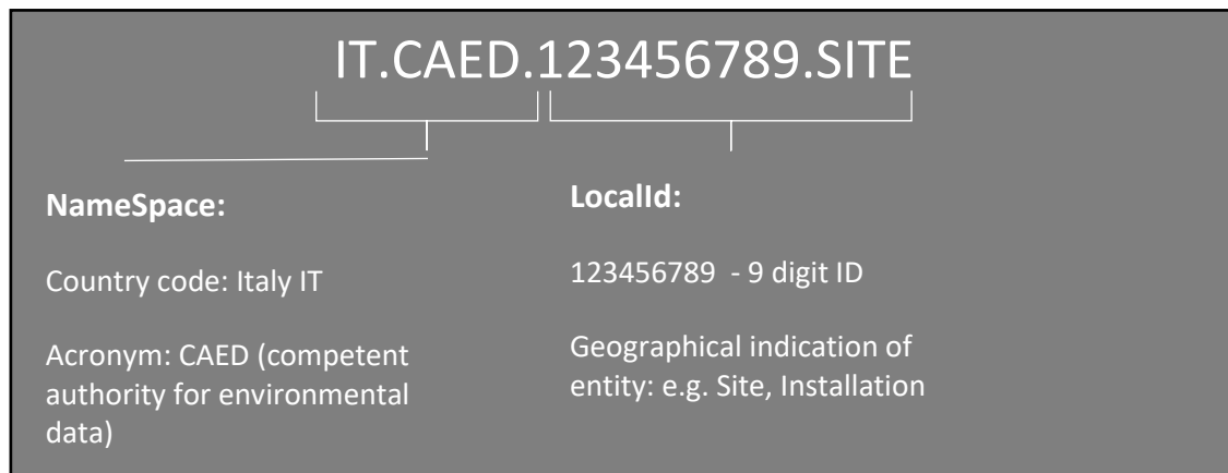
Figure 5 - An example inspireId broken into its components.
